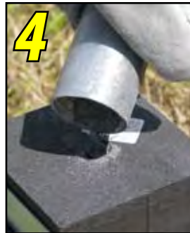
Place a small amount of starting powder in the ignition pocket.
